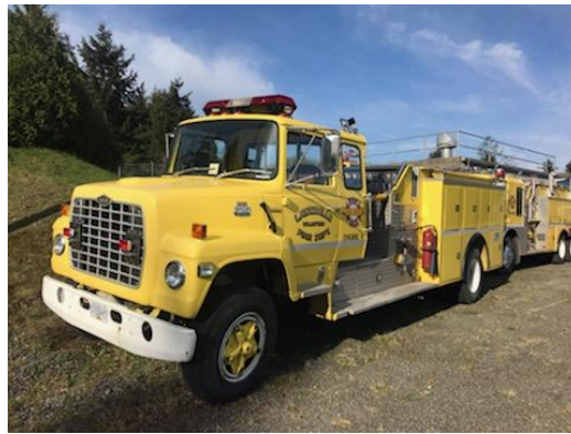
1981 Ford Fire Truck (Fire Truck #4) 3208 Cat Diesel V8 4-speed Allison Automatic, 850 gpm pump
