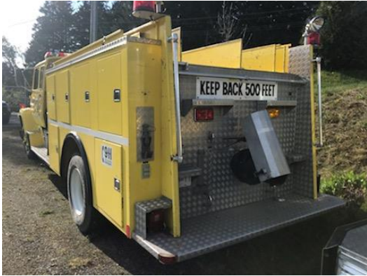
1981 Ford Fire Truck (Fire Truck #4) 3208 Cat Diesel V8 4-speed Allison Automatic, 850 gpm pump
